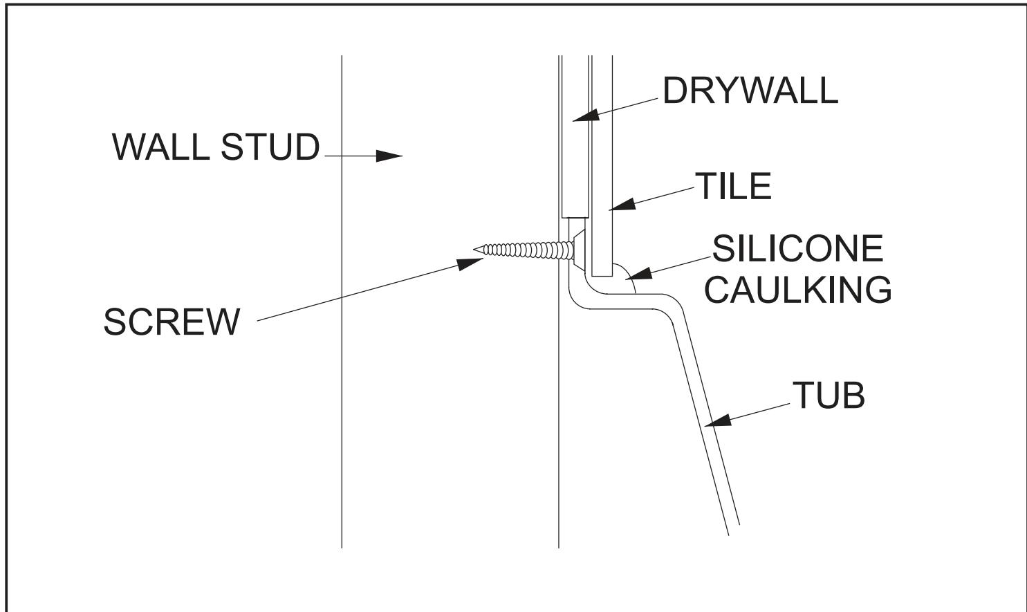
Apply silicone and remove the protective film as shown below.
