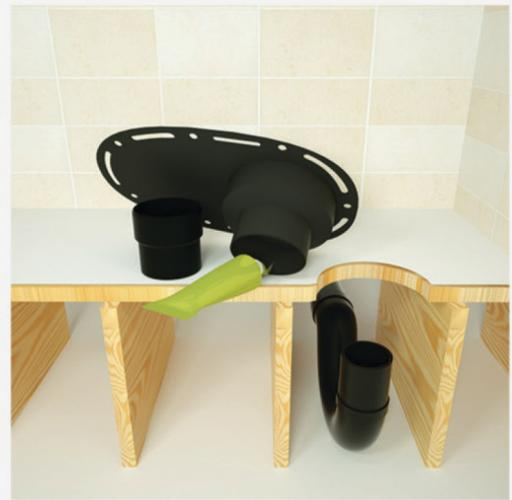
**2.** Measure and cut a ABS or PVC piece as needed to ensure a secure connection with the P-trap below. Note that the drain body has an outlet of 2" (a coupling reducer of 1 1/2" is included).
